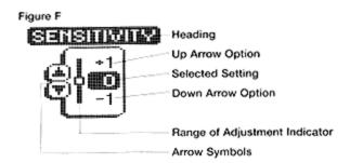
If no adjustment is made, this will be the selected setting. Pressing one of the ARROW buttons while the menu is on-screen selects another option.
